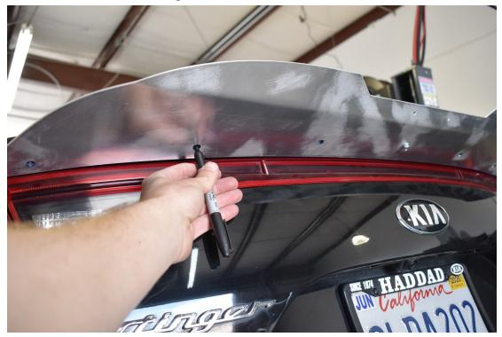
9.) Remove the spoiler extension, drill the holes  $\frac{1}{8}$ ", then 25/64", then install rivnuts into each hole.
