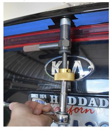
7.) Install your spoiler extension onto the center rivnut using a countersunk bolt and washer.
