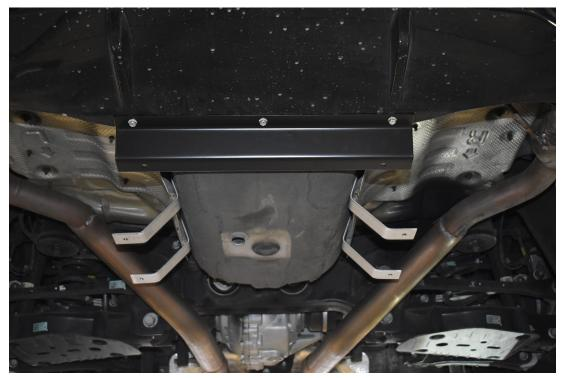
6.) Install your diffuser! Install it onto the rear "s" bracket first with M6-1.0 x 20mm bolts pointing upward with 1" OD fender washers under the heads, and  $\frac{1}{4}$ " small washers + nyloc nuts on top. Securely tighten.
