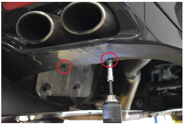
10.) Install your outer pieces into those holes just exposed from steps 8 and 9. The clips are replaced with M6-1.0 x 20mm bolts with 1" OD fender washers under the heads, and  $\frac{1}{4}$ " small washers + nyloc nuts on top. The 10mm bolts that were removed from step 9 are replaced with M6-1.0 x 20mm bolts with  $\frac{1}{4}$ " lock washers and 1" OD fender washers under the heads. Securely tighten.
