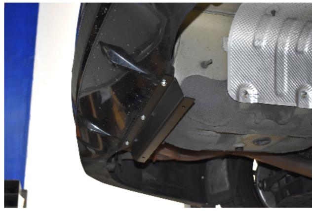
4.) Identify and remove the 10mm bolts found on the left and right sides of the trunk bottom.
