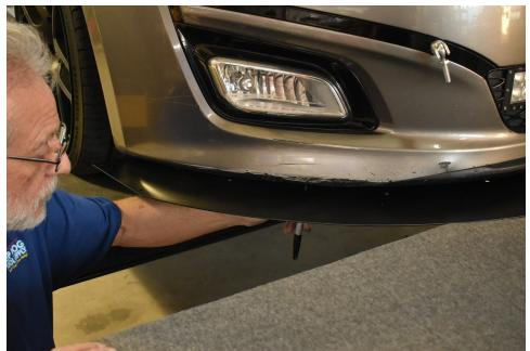
7.) Once the holes have been marked remove the splitter. If you need to... drill out the holes. Then, locate where you want to place the splitter rods. Splitter rods come with their own instructions/recommendations. We are just here to show you where we located ours. Rods should be installed onto the bumper/car <u>before the splitter is installed</u>. The picture below shows that the rods were installed onto the car about 3 5%" from the front grill.
