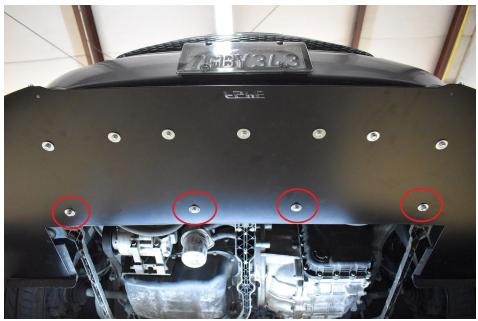
10.) Use your 1/4" bit to drill through the remaining 2 holes in the splitter into the car. Install in the same manner as the bolts found around the perimeter on the bumper.
