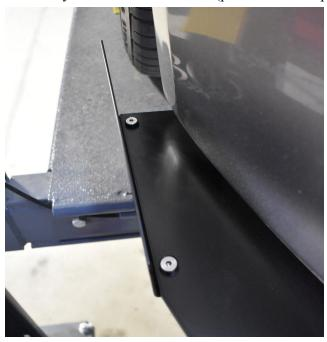
13.) Install your rods into the 2 front holes. If you have a 3 piece, the rods mate the splitter together. Use the supplied splitter rods installation instructions to assure it is installed correctly.
