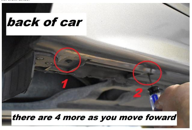
3.) Install your side skirt into these screw holes. We supplied both 1" body screws, and 1.25" long body screws. Use two longer body screws for the rear holes/slots (location shown in previous step) and the 1" body screws for the 4 holes in the middle and front.
