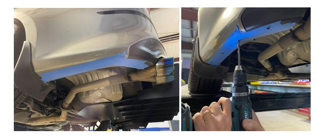
11.) Drill the marked holes in your outer pieces. Install your outer pieces. The hole toward the back of the car uses a M6-1.0 x 20mm bolt. The remaining holes use M6-1.0 x 40mm bolts and **15mm spacers**. Use nyloc nuts on top, large washers on bottom, and small washers on top. Securely tighten.
