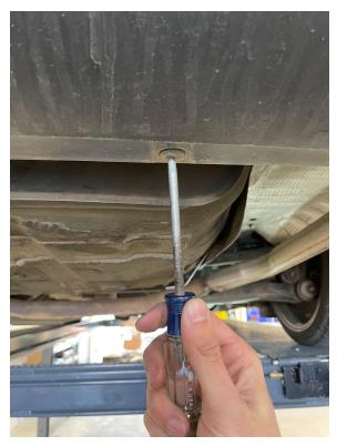
6.) You can now install your center diffuser with help from a friend. At the rear the diffuser installs into the holes from the previous step. You will need to use a M6-1.0 x 45mm bolt and nyloc nut on top. A 20mm spacer needs to be placed between the diffuser and bumper. Use large washers on bottom, and small on top under the nut. Leave loose.
