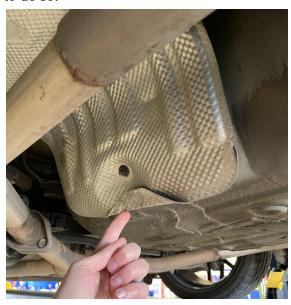
3.) Identify and remove the nut on each side of the car holding the head shield.
