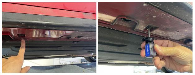
7.) You can now install your side skirt extensions in the holes (again, 5 on each side). Use the supplied M6-1.0 x 16mm bolts with 1" OD washers on bottom, and  $\frac{1}{4}$ " small washers + nyloc nuts on top. Tighten securely.
