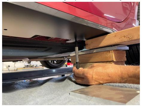
5.) Once the holes are marked, remove the side skirt extensions. Use a drill and ¼" drill bit to drill through the plastic rocker panel. There should be 5 holes on each side.
