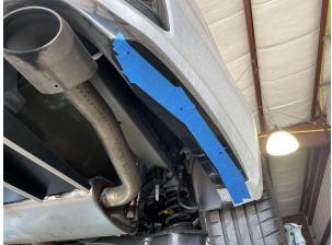
6.) Drill 1/4" holes in the bumper where the marks were made, then remove the tape.
