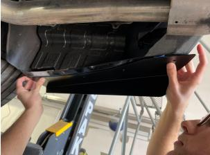
5.) Hold the spat firmly and mark the spat's holes onto the bumper. Remove the spat and make sure the marks are on the flat surface of the bumper - not too close to an edge. If they are, remark. See where we placed ours.
