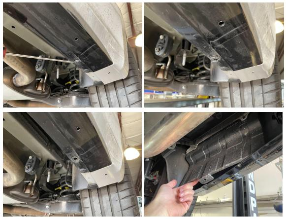
8.) Install your spat. Use the supplied bolts pointing upward. Place the larger washers on bottom, and small washers above the bumper with nyloc nuts. Mount securely.
