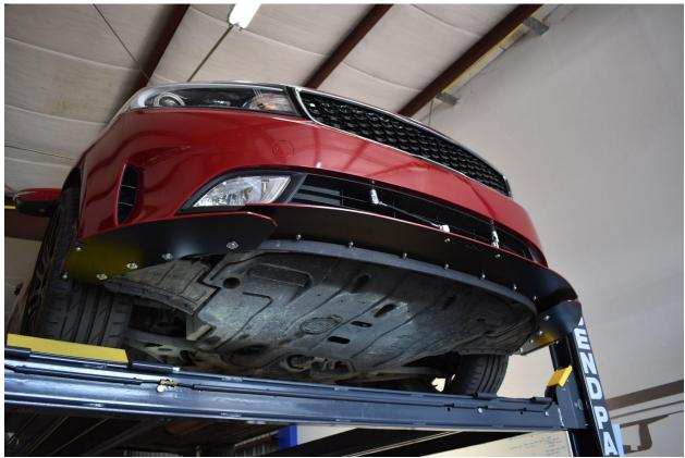
12.) If you have edge trim, prep the surface edges with isopropyl alcohol and apply the trim. Use a heat gun or hair dryer if you need to form the edges around corners.
