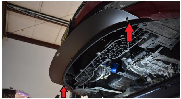
5.) You can now drill through the remaining holes in the center splitter piece. Remove the center bolt. Then install M6-1.0 x 20mm bolts UPWARD with  $\frac{1}{4}$ " small washers and M6 nyloc nuts on top. After that, remove the outer two M6-1.0 x 20mm bolts / whiznuts so the outer holes are empty.
