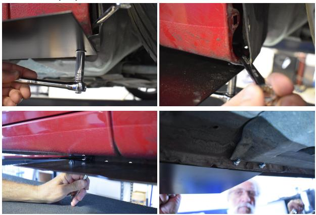
9.) Reinstall the clip and screw just behind the front tire into the fender well.
