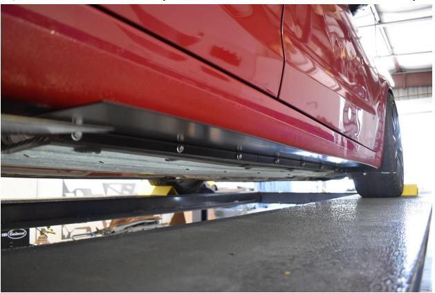
14.) Install your winglet using the countersunk hardware. Use oil on the threads when installing.
