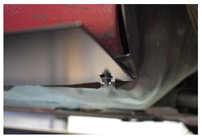
7.) Level the piece and mark through the holes in the side skirt piece onto the jack point rail. Assure the bottom of the side skirt piece is above the bottom of the rail so you can still jack up the car. Then remove the piece and use a ¼" drill to drill through the holes just marked in the rail.
