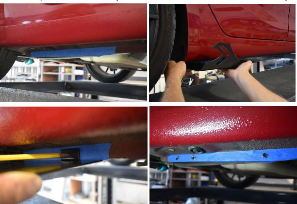
11.) Install your rear side skirt piece using M6-1.0 x 20mm bolts and M6 nyloc nuts.
