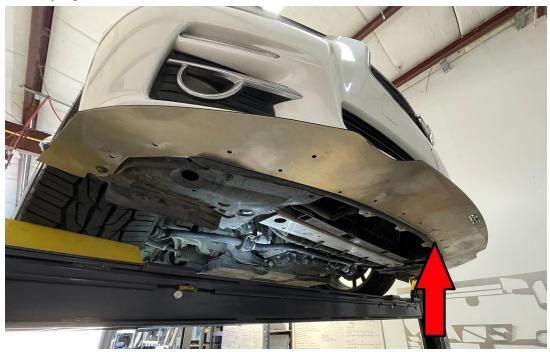
6.) Drill out the remaining holes through the bumper with your ¼" drill bit.
