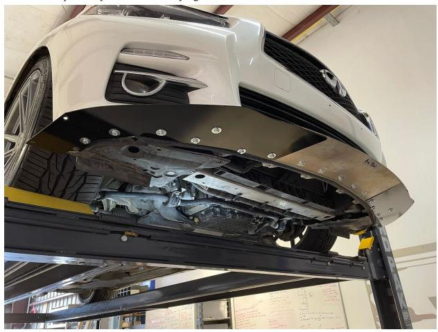
8.) Install your fins. Use a little bit of oil on the threads of the bolts since they are stainless steel. Use the countersunk hardware with the ¼" small stainless steel washers and nuts on bottom. Don't over tighten.
