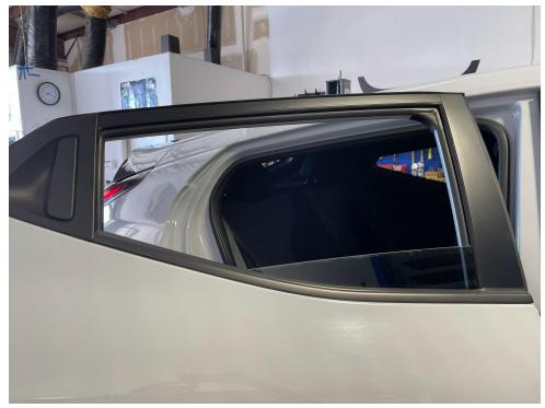
2.) In the vent the top side toward the back of the car has a small hole in it. Slip the window vent into the window slot by inserting it at the rear first, then slipping it upward. DON'T BEND THE PIECE TO GET IT INTO THE SLOT.
