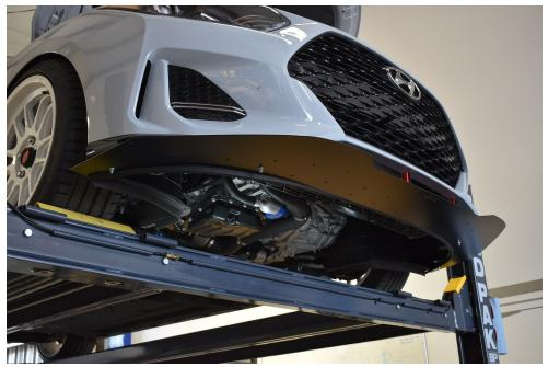
16.) Drill up through the remaining holes in the splitter. Then fill them with the same nut/bolt combo. Lay the 2nd splitter layer underneath the top layer in the center. Note 1: BE SURE NOT TO DRILL PAST THE 1ST LAYER IN THE BUMPER - don't allow the drill to push up and drill into the upper bumper. Note 2: blow out the plastic residue made between the splitter and bumper before installing the hardware. Securely tighten these bolts.
