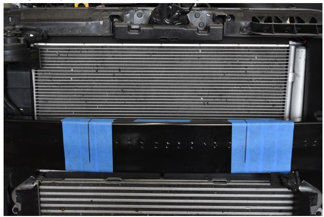
8.) Align the holes in your brackets with the vertical lines. Use a level at the top to assure it's flush with the top of the beam. Then mark your holes.
