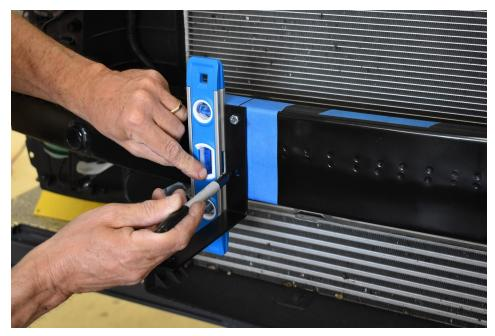
9.) Now that the holes are marked, use your  $\frac{1}{4}$ " INDUSTRIAL DRILL BIT to drill through the crash beam. Assure you are drilling perpendicular to the beam. Drill through both the front and back of the beam so a bolt can pass through both sides. Total holes drill = 8.
