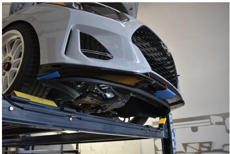
13.) Elevate the splitter up against the bumper. Wooden blocks and a friend should do the trick. The splitter should sit against the black "flap" found behind the underside of the bumper. (FIRST PIC SHOWS THIS). Maneuver the splitter so it is symmetrical. This means that it sits at the front of the inner fender well equally on both sides of the car. Mark up through the outer holes and center hole with a sharpie onto the bumper. (2nd PIC).
