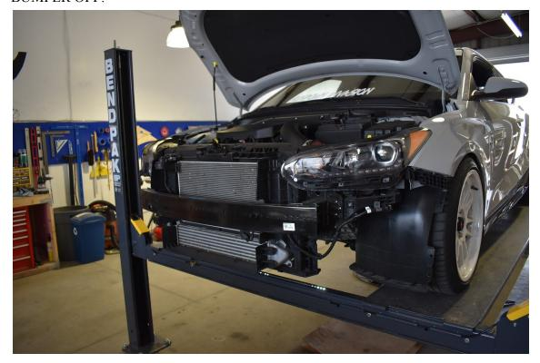
6.) Now that the bumper is off, locate the black bash/crash bar. Find the center of it using your flexible measuring tape - lay down masking tape and mark the center with your marker. Then place tape approximately 5-7" to the left and right of the center mark.
