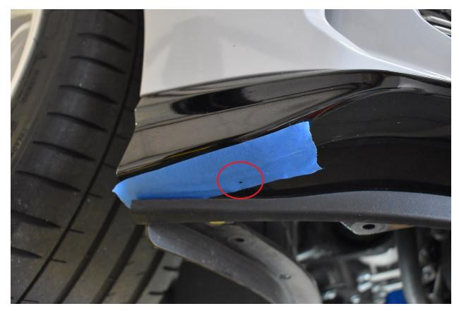
14.) Now that you've marked a couple of the holes onto the bumper, remove the splitter and drill through them with your drill and  $\frac{1}{4}$ " drill bit.
