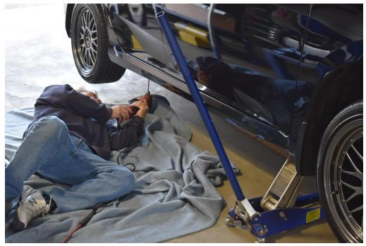
5.) Remove three of the clips that hold the rocker panel onto the car (underneath the rocker panel). There are four but you only need to remove the rear three. First pic shows what the clip looks like, second is an example location.
