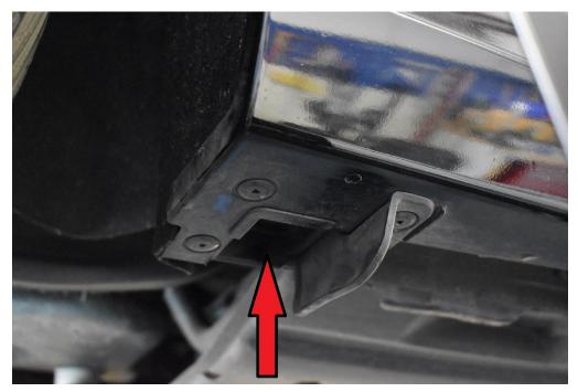
6.) Once the clips are removed, install a side skirt into the holes you made (they are symmetrical). One of the holes can be seen in the picture above!! Use the M6-1.0 x 20mm bolts pointing upward with 1" OD fender washers under the heads, and ¼" small washers + nyloc nuts on top. Tighten all bolts/nuts securely.
