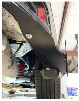
8.) Use your <sup>1</sup>/<sub>4</sub>" drill bit to drill through the 3rd hole in the diffuser into the bumper. Then install a M6-1.0 x 20mm bolt with the same washer/nut combo as the previous step. Securely tighten.
