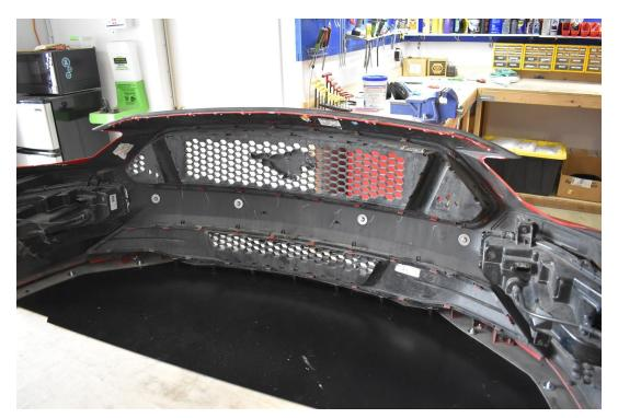
13.) Reinstall your bumper. You no longer use the OEM skid plate. After it is installed you will need to bolt it to the frame. We supplied long bolts and washers to do so. Use the M6-1.0 x 55mm long bolts toward the front of the car (green circles) and M6-1.0 x 60mm bolts (red circles) toward the back. Use the 1.25 outer diameter washers on top and bottom, and nyloc nuts on top. It will be a tight squeeze. See pictures.
