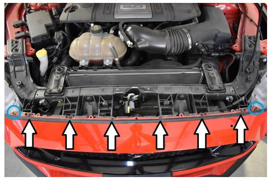
4.) Remove the skid plate. The skid plate is held on with 21 screws (7mm head) and 4 clips (use your flat head screwdriver). The screws are circled in red. Two of the clips at the rear (arrow) and two are found at the fender well (1 on each side, arrow).
