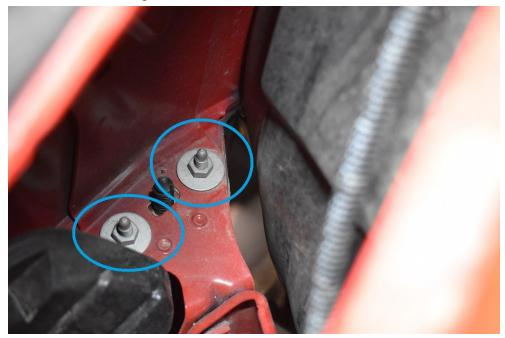
8.) The bumper can now be pulled off with help from a friend. The outer edges need to be pulled outward away from the fender and headlight, and the center lifted over the pins that hold it. While pulling it off unplug the fog light electrical clips. We placed our bumper on our table while doing this.
