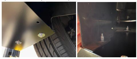
9.) Install the brake cooling ducts with <u>M6-1.0 x 20mm</u> bolts, NO washers, and m6 nuts.
