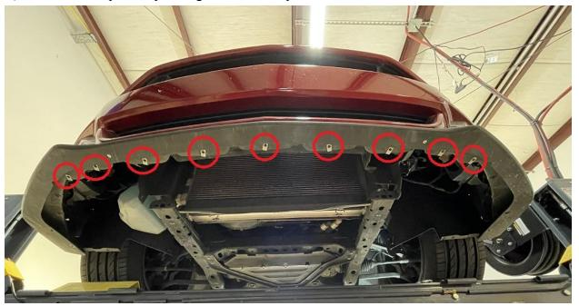
4.) If you have splitter rods, install them into the bumper now. Use the supplied rod instructions for help. The rods need to be installed into the bumper before the splitter can go on. Here is where we put ours.
