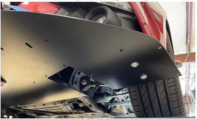
6.) Install  $\underline{\textbf{M6-1.0 x 30mm}}$  bolts into the center 9 holes where the speed nuts were removed. Use 1" fender washers on top and bottom + nyloc nuts on top.
