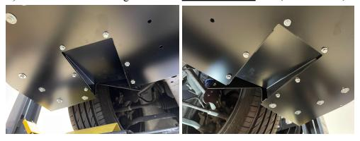
10.) Install your chassis bolts. Use the longer <u>M6-1.0 x 55mm</u> bolts supplied with 1.25" OD fender washer below the splitter, and on the chassis. The bolts pass through both holes in the chassis.
