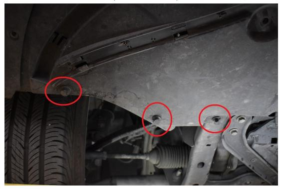
3.) Remove the 6 speed nuts found along the front of the bumper with a flat head screwdriver or needle nose pliers (or other useful tool).
