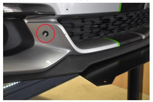
9.) Install your outer splitter pieces onto the car into the OEM holes with six M6-1.0 x 20mm bolts and six whiznuts - just to hold it all in place. Use a provided 5/16"-18 splitter bolt to hold the front holes in the splitter together.
