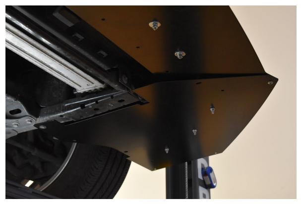
10.) Use one of the OEM pop clips on each side at the rear of the outer splitter pieces to help hold it in place.
