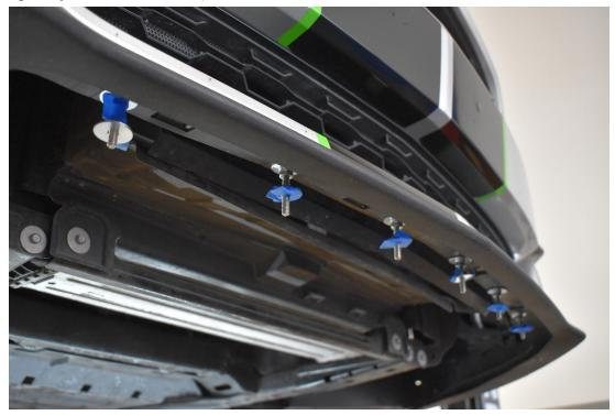
7.) Install your center splitter onto the middle four all threads with  $\frac{1}{4}$ "-20 nuts,  $\frac{1}{4}$ " lock washers, and 1" OD fender washers. Just snug for now. Remove the tape if you want on these 4.
