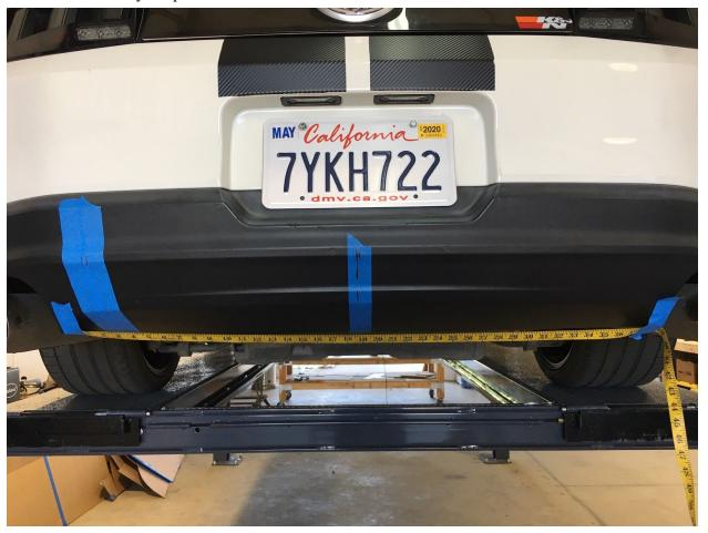
3.) Hold your center fin up to the car. This fin will be marked. With help from a friend hold the fin perfectly in parallel, or straight, with the car. Feel free to use the measuring tape to your advantage. Use your pen to mark through the holes onto the tape. Be sure the fin contours the rear valence as best as possible. See pics.
