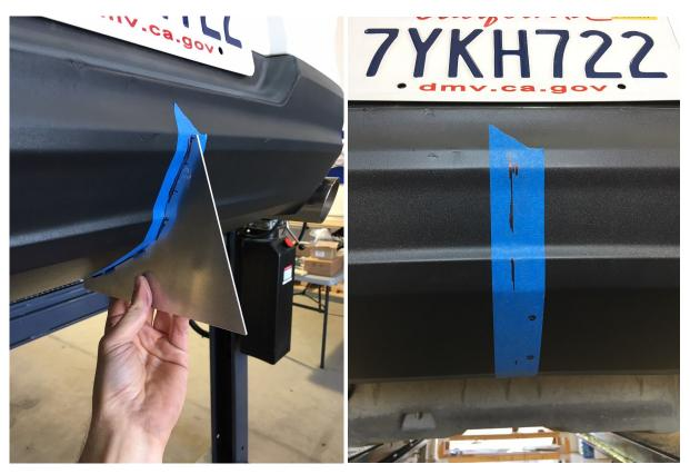
4.) Use your ¼" drill bit to make holes where you marked. Remove the tape. Then install your center fin with the countersunk bolts and washers on the outside, and ¼" small washers and nuts on the inside. Tighten securely.
