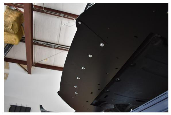
5.) Find the locations where holes need to be drilled into the bumper. These are where holes are not already present in the bumper. Use your ¼" drill bit and drill to make the holes. There should be two locations on each side of the bumper.
