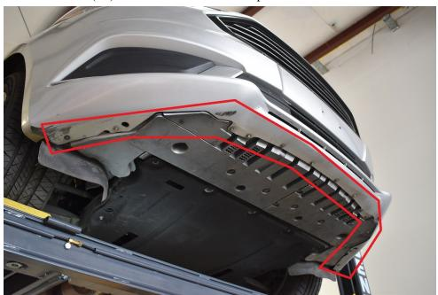
→ Remove the (3) 7mm screws on each side (so a total of 6) that hold the fender well.
