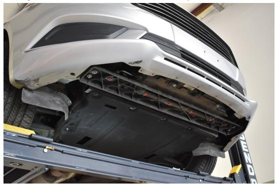
3.) We recommend finding a location to mount your splitter rods. We mounted them in the area pointed to, and also think the area to the right circled will work just fine as well. Mount them to the car first before installing the splitter. Feel free to test fit the splitter first to find a location. Use the supplied splitter rod installation guide for tips and guidance.
