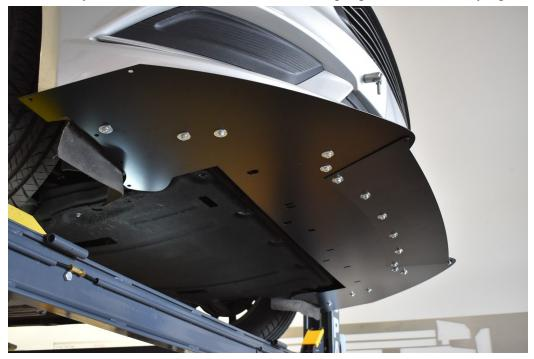
7.) Now install 1" body screws into the 3 holes onto each side that hold the fender liner. Don't over tighten, they are just there to keep things in place. We only installed 2 on each side in the picture - sorry not sorry.
