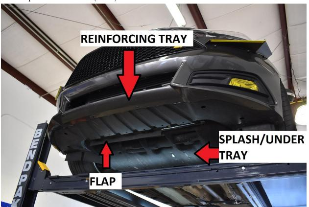
3.) Remove 4 of the red clips that hold the trays to the chassis using your needle nose pliers. We just used our fingers. We recommend removing 4 clips that don't hold your OEM splash tray up leave those ones on.
