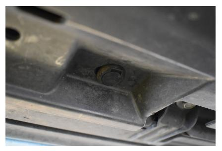
3.) After removing those clips, the entire skirt will be able to "pop" off of the clips attached to the rocker panel. The skirt sits on these clips. Start toward the back of the car and pull the skirt away from the car, while also pulling upward. Pop the skirt out of each individual clip while moving toward the front of the car. The skirt at the very front shouldn't be "popped" out, just pulled toward the back of the car.
