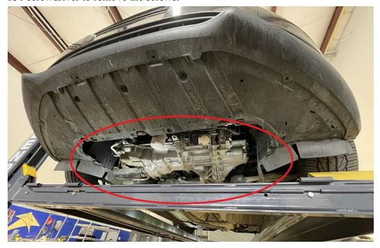
3.) Remove the undertray that sits on the bumper and aluminum rail. This undertray will be entirely replaced by the splitter. There are 6 populips circled in green, and 7 T30 screws circled in red. There might be 3 more screws/populips where the blue square is (ours were missing).
