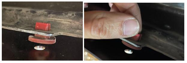
Here's what the splitter bolts look like once installed: Remember to remove all red clips.
