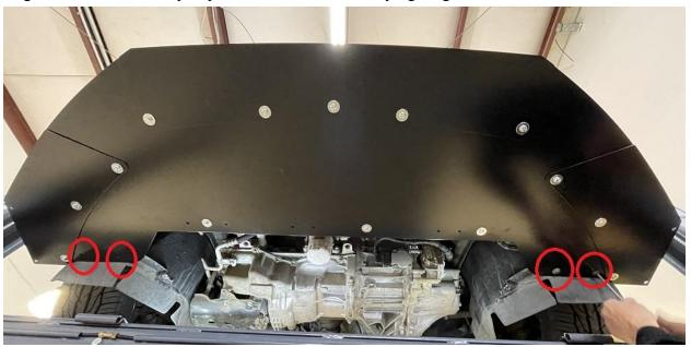
10.) Reinstall the splash tray. Use the same nut/washer/bolt combo for the front 3 (pass through the splitter as well), and OEM screws for the remainder of the holes.
