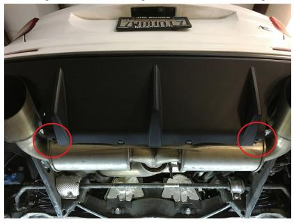
7. Insert the remaining short length (3 1/4") threaded rods into the holes according to the picture in step 3. In this case the "RS Frame" from the picture in step will be the plastic, metal, and metal clip. Note: yours will have the lock washers (picture does not). Also note there is no specific length determined for this threaded rod - you need to adjust it so the diffuser fits under the exhaust. Hand tighten for now.
