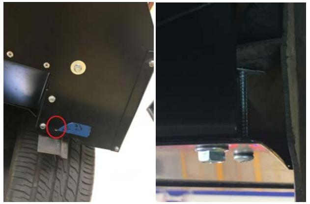
13.) If you haven't already for the splitter V1, drill 5/16" holes into your splitter where you want to mount your support rods. Then mount your support rods. Be sure to use blue threadlocker on the bolt threads (NOT THE HEIM JOINT THREADS).
