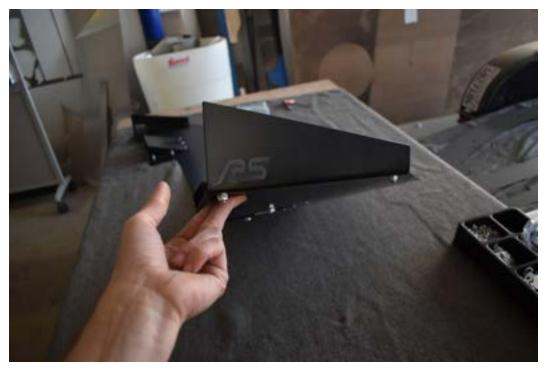
6.) Install the air ducts on the splitter using M6-1.0 x 20mm bolts pointing upward with nyloc nuts on top. Ignore the pop rivets in our picture - you will have bolts.
