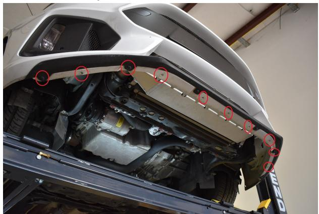
Splitter secured on bumper but not rear chassis:
