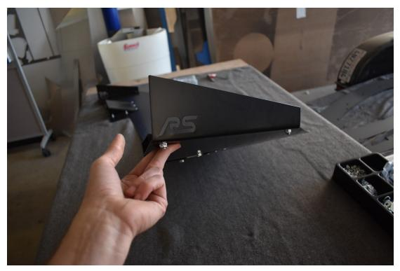
6.) Install the air ducts using M6-1.0 x 20mm bolts pointing upward with nyloc nuts on top. Ignore the pop rivets in our picture - you will have bolts.
