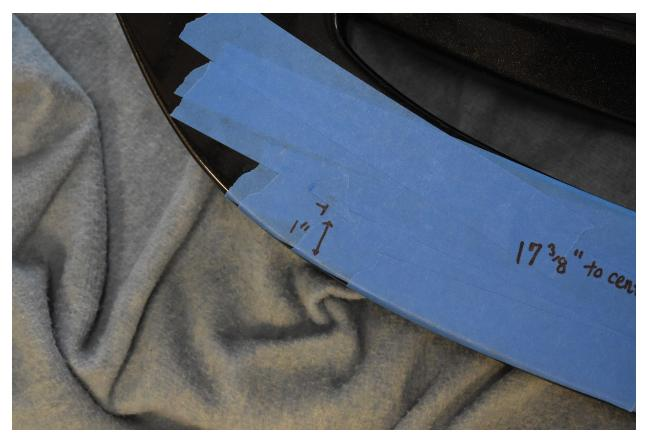
6.) Once we were confident the spoiler was centered, we drilled  $\frac{1}{8}$ " holes into the outer two marks. Then opened them up to 25/64".
