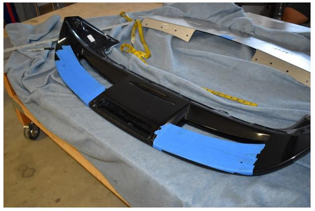
3.) Center the spoiler. Place tape onto the center of the underside of the spoiler extension, and mark the center (pic 1). Then use the center indicator on the OEM spoiler to center the spoiler. The center indicator is shown in the second picture - middle of the two lines.
