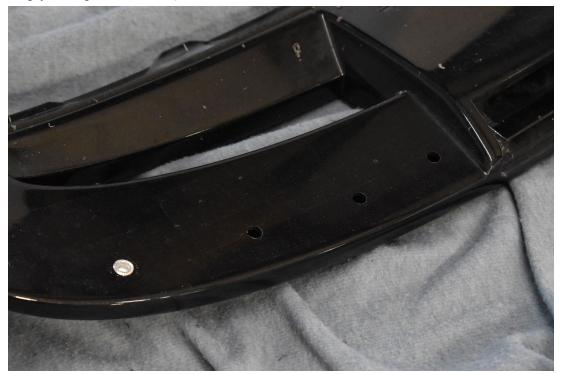
8.) Install your spoiler extension onto your OEM spoiler into the outer two holes. Use the hardware supplied. Then mark the 6 remaining holes.
