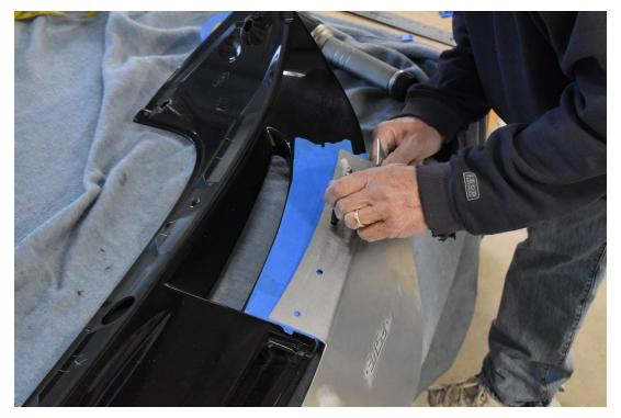
9.) Remove the spoiler extension and drill out the holes just marked with your ½" then 25/64" drill bits. Then remove the tape and install rivnuts into each hole. You should have a total of 8 rivnuts installed. Like this!! (OURS WAS ON THE CAR, IGNORE THAT!!!!)
