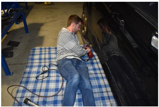
6.) Once the holes have been drilled you can now install your side skirt. Use the M6-1.0 x 20mm bolts pointing upward with 1" OD fender washers under the bolt heads. On the top of the OEM rocker panel use \(^{1}\_{4}\)" small washers and nyloc nuts.
