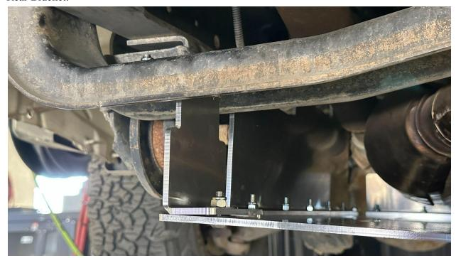
6.) Install your main plate directly onto the transmission's crossmember at the location shown. Use a 5/16"-18 x 6.5" bolt, 5" spacer, and 5/16" nyloc nut. There are THREE 5/16x1.25" washers that need to be used: 1 under the bolt head, 1 under the transmission crossmember but above the spacer, and 1 on top of the crossmember under the nut. Securely tighten.
