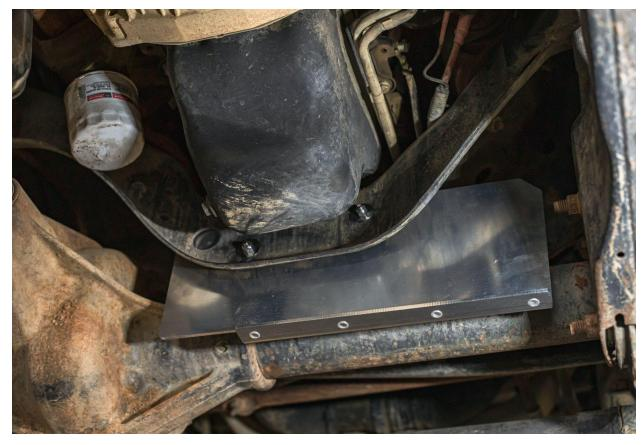
4.) LOOSELY install your rear "z" bracket as shown onto the transmission crossmember using ONE 5/16"-18 x 1" security bolt and 5/16" nyloc nut. Use 5/16x1.25 washers on top and bottom.
