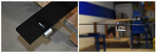
4. While a friend holds up the back end of the side skirt, line up the bracket and skirt on the car on the pinch weld so the skirt is flush with the front of the rocker panel. Bring the bracket hole as low as possible, leaving room for the hole you will drill, and make a mark on the pinch weld with your sharpie. You might have to move the plastic pieces from step (2.) out of the way. Feel free to use masking tape so the sharpie shows up better against the rails.
