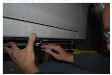
7. Install the 3 remaining brackets onto the skirt. Mark the holes for the rest of the brackets onto the pinch weld, remove the skirt, and drill out each hole. Reattach your side skirt onto the car and securely tighten each 10-24 bolt/nut. Finally adjust your side skirt so it is where you want it and securely tighten each M6 bolt/nut with your 10mm wrench. Use needle nose pliers to hole the threads on the bolt while tightening the nut.
