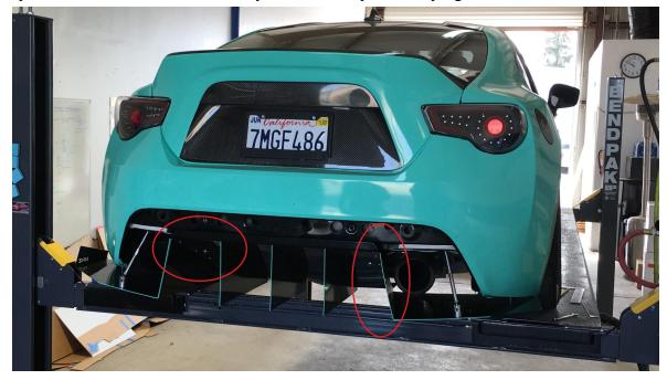
9.) Install the diffuser into the holes exposed from step 7. In the hole toward the front of the car use a M6-1.0 x 20mm bolt & 1" OD fender washer on bottom, a 5mm spacer between the diffuser and car, and a 1/4" small washer & nyloc nut on top.
