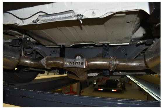
5.) Identify these two holes in the rear subframe and <u>loosely</u> install your short brackets. Use 20mm bolts toward the back of the car, and ½" small washers and nyloc nuts on the other side.
