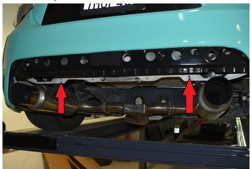
3.) Identify and remove the two front-most bolts that secure the rear muffler exhaust shield. You will <u>not</u> be reusing these bolts.
