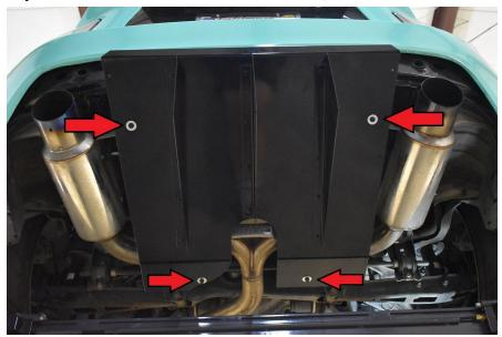
7.) Remove the 1 to 2 clips toward the front of the car that can be found at either end of the rear bumper. Yours will likely have two, not three. We want to use the two holes circled in the pic. We later realized these clips hold some kind of boxy bumper support (as can be seen). Feel free to work around the box by cutting the fins on it, or just remove it all together (recommended).
