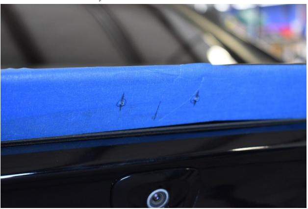
5.) Use your 25/64" drill bit to open up the holes. Then remove the tape around just those holes.
