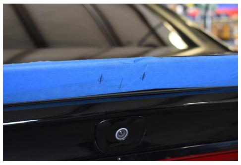
4.) Check that the two holes are spaced upward equally from the bottom of the trunk. Double check fitment a few times by lining up the wickerbill on the OEM spoiler. Once you are confident that the two holes are correct, drill them out with your small drill bit (~½"). FOR ALL HOLES BEING DRILLED BE SURE NOT TO GO THROUGH THE OEM SPOILER AND HIT THE OTHER SIDE. Take your time!!!
