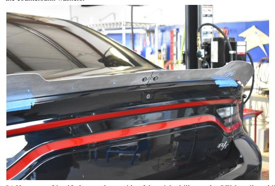
8.) Have your friend/helper push one side of the wickerbill onto the OEM spoiler while you push the other side. Assure the wickerbill is positioned at the same spot on both sides of the OEM spoiler. If it is not, loosen the center two bolts and adjust accordingly, then retighten them and push both sides of the wicker bill. Mark all of the remaining holes.
