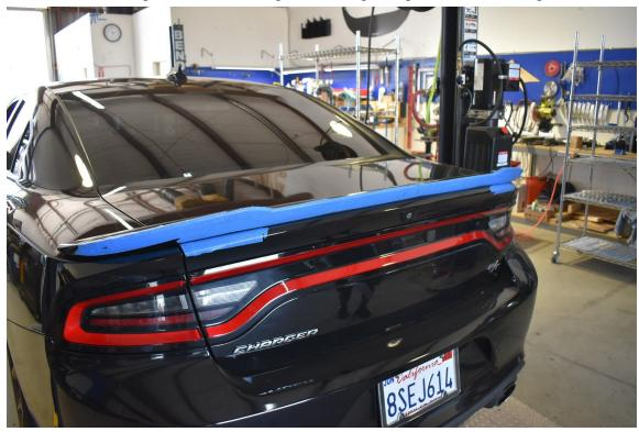
2.) Use your measuring tape to find the center of the wicker bill. The reverse camera is centered as well so feel free to use a level to locate the center of the wickerbill. Then mark the center.
