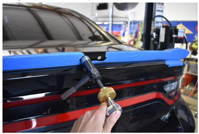
7.) Install the wickerbill onto the OEM spoiler by threading two of the bolts into the rivnuts. Use the countersunk washers.
