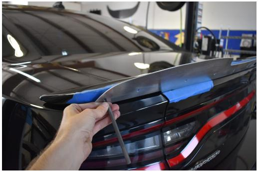
9.) Once all holes are marked, remove the wickerbill. Drill out each hole with your small drill bit, then with the larger 25/64" bit. Then remove tape and install rivnuts into each remaining hole. Our test wickerbill has a lot more holes than yours! Don't worry about that:)
