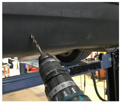
6.) Install your center diffuser into the two holes just drilled. Use  $\frac{1}{4}$ "-20 x 1.25" long bolts and countersunk black washers upward - *place a 10mm spacer* between the diffuser and valance for both holes. Use  $\frac{1}{4}$ " stainless washers and  $\frac{1}{4}$ "-20 nyloc nuts on the inside. Tighten securely.
