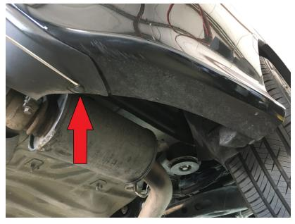
14.) Place blue tape on the underside of the bumper just behind the tires. Then install the outer pieces into the hole from the previous step. Use  $\frac{1}{4}$ "-20 x 1" countersunk bolts & countersunk washers on bottom, and  $\frac{1}{4}$ " washers and  $\frac{1}{4}$ "-20 nuts (NOT NYLOC) on top. Hand tighten.
