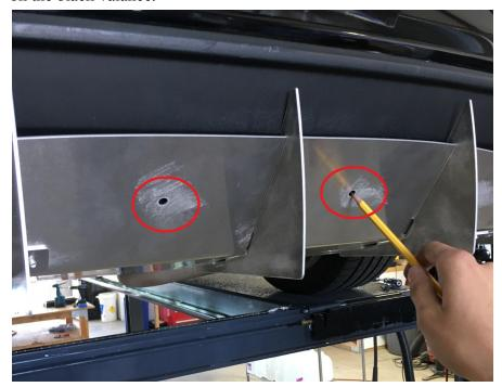
5.) Remove the diffuser from the car and drill the holes just marked. Only go through the valance. Use a  $\frac{1}{4}$ " or  $\frac{5}{16}$ " drill bit.
