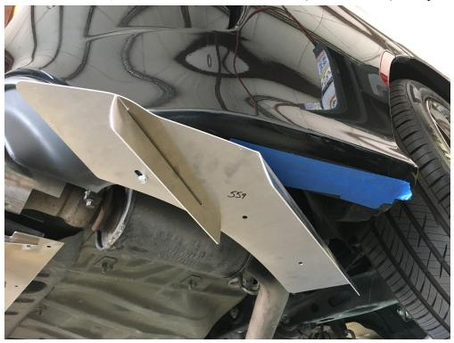
15.) Rotate the outer pieces so they are flush with the fender well and mark the holes onto the masking tape.
