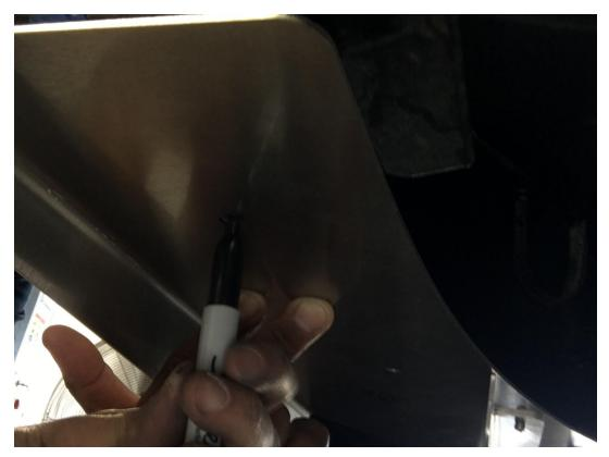
16.) Remove the outer pieces, then drill the holes with a  $\frac{1}{4}$ " or  $\frac{5}{16}$ " drill bit. Then remove the tape.
