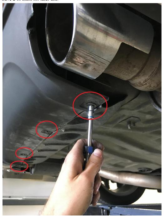
3.) Install the center diffuser into the outer two holes of the OEM valance. Use the  $\frac{1}{4}$ "-20 x 1" countersunk bolts & black countersunk washers pointing upward, and  $\frac{1}{4}$ " stainless steel washers & nuts (NOT NYLOC) on top. Leave hand tight - center the bolts in the slots.
