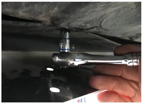
8.) Install  $\frac{1}{4}$ "-20 x 1" countersunk bolts and countersunk washers into the outer two holes in the valance. Use  $\frac{1}{4}$ " stainless steel washers, and  $\frac{1}{4}$ "-20 nyloc nut - securely tighten. The center is done!!!!
