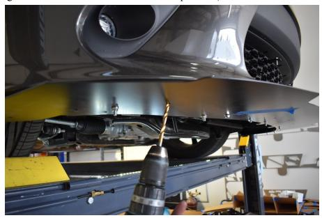
6.) Remove the splitter. Then remove the undertrays all together. The front undertray has those 8 bolts around the front that we already removed previously, and 10 additional pop clips in various locations. The rear tray has four 10mm bolts. Please remember how everything goes back on. HERE IS HOW WE REMOVE THE CLIPS:
