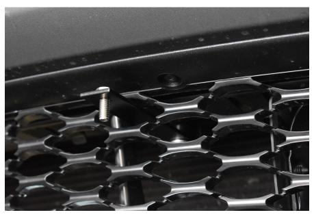
16.) Splitter install. Install the splitter into the holes that you drilled, and the 4 holes from step 2. You want to leave the 8 holes from steps 3 and 4 open. Use M6-1.0 x 20mm bolts with 1" washers under the heads, and \(^1/4\)" small washers and nyloc nuts on top. Securely tighten. HERE'S THE CATCH:
