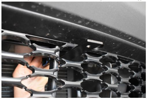
9.) Start by placing a 20mm spacer onto your chassis bracket. Tape it down directly over the hole closest to the fold.
