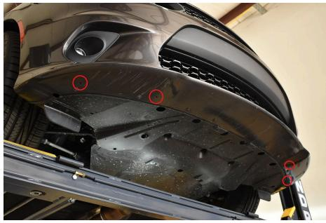
3.) Remove the 8 screws around the perimeter of the bumper & store them away, they are no longer needed. These screws hold the undertray onto the front bumper. Use your 7mm wrench.
