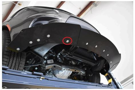
9.) Reinstall your under trays. The front under tray will be using the  $1-\frac{1}{8}$ " long body screws into the remaining holes in the splitter. Make sure everything is securely tightened.
