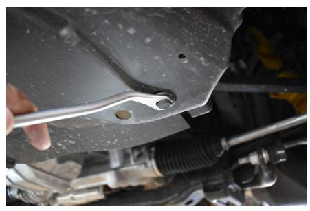
HERE ARE FOUR CLIPS FOR THE FRONT UNDERTRAY (they point upward)
