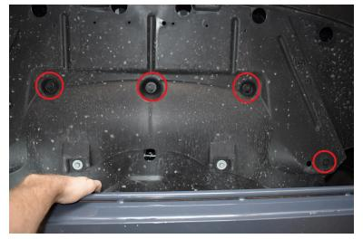
HERE ARE THE 3 CLIPS ON EACH SIDE THAT NEED TO BE REMOVED (just in front of the wheels):
