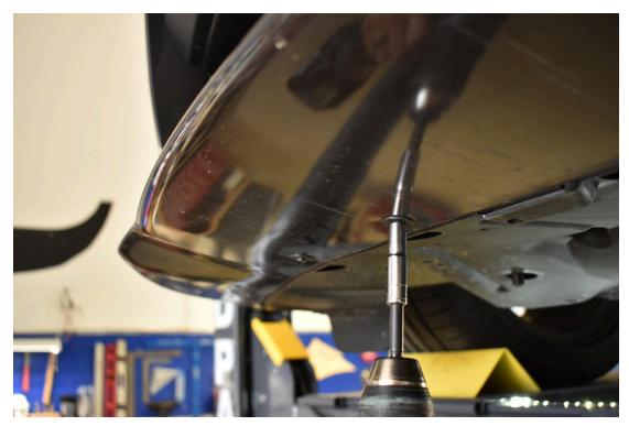
4.) Install the top layer splitter (not the smaller bottom layer pieces) into those holes just exposed from step 3. Don't use the OEM screws. Use the supplied  $1-\frac{1}{8}$ " long body screws supplied in the kit.
