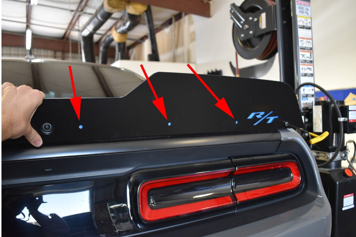
7.) Mark the remaining holes through the wicker bill and onto the OEM spoiler - a total of 6.
