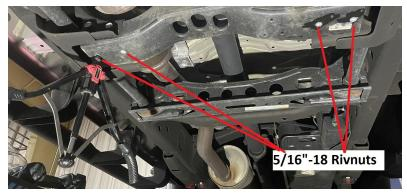
6.) Located the OEM hole in the rear bracing on the vehicle located on the passenger side. There will be two holes. Drill out the rear hole with a 25/64" drill bit and install a ½-20 **SHORT** rivnut.
