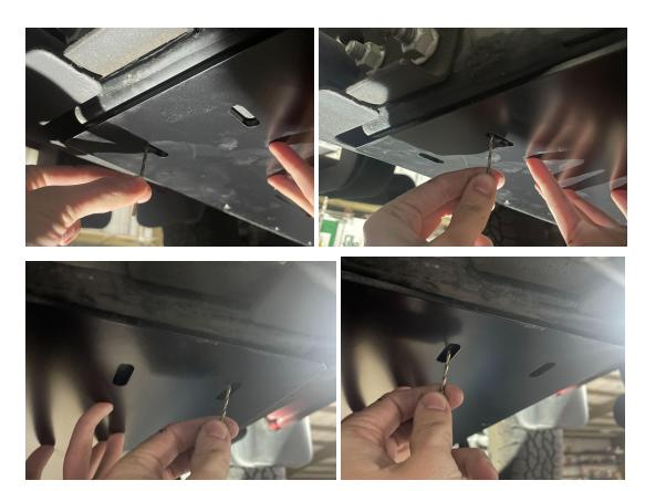
5.) Once you have all 4 of the slots marked, remove your cat guard. Then at the center of each slot drill a 17/32" hole and install the 5/16"-18 rivnuts.
