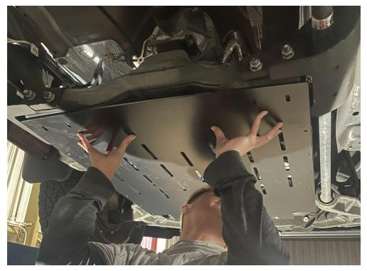
4.) Position the back end of the cat guard against the rear crossmember that supports the transmission. Align it so the same amount of guard hangs off the crossmember on the left and right sides. Align the front end of the cat guard so the bolts are centered in the slots (front-to-back). Use a marker (we used the end of a drill bit) to mark the 4 slots onto the crossmember.
