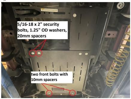
8.) Now install the rearward shield simultaneously. It sits on top of the cat guard using two of the common holes on the right side. Use 5/16"-18 x 2" long security bolts, 1.25" OD washers, and 20mm spacers. **Hand tighten.**
