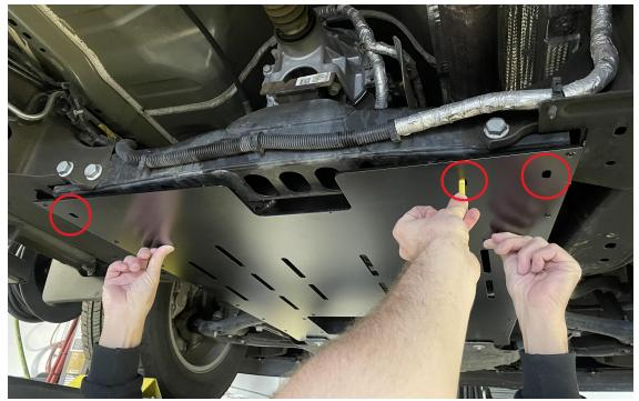
5.) Once the marks are made on your rear transmission crossmember, remove the guard. Drill out 17/32" holes where the three marks were made. Feel free to start with a small drill bit and work up to a 17/32".
