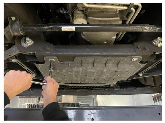
3.) Install your cat guard above the skid plate using the bolts just removed - tighten only snug.
