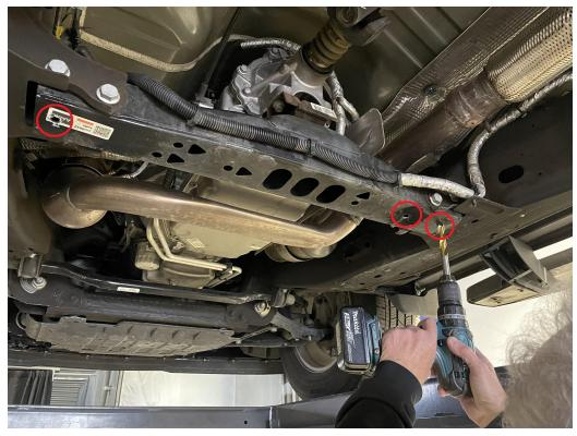
6.) Install 5/16" rivnuts into the 3 holes just drilled. Need help? See the first page and scan the QR code.
