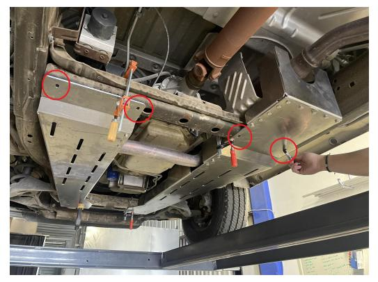
5.) The cat guards can be installed in two ways. You can install the 5/16"-18 rivnuts into all of the holes for mounting, OR you can install rivnuts into the CENTER REAR TWO holes and then bolt/nut combination into the remaining six holes.
