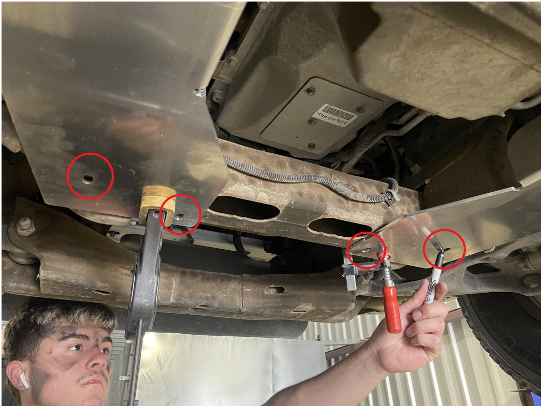
4.) Mark the 8 slots in the cat guard onto the frame.
