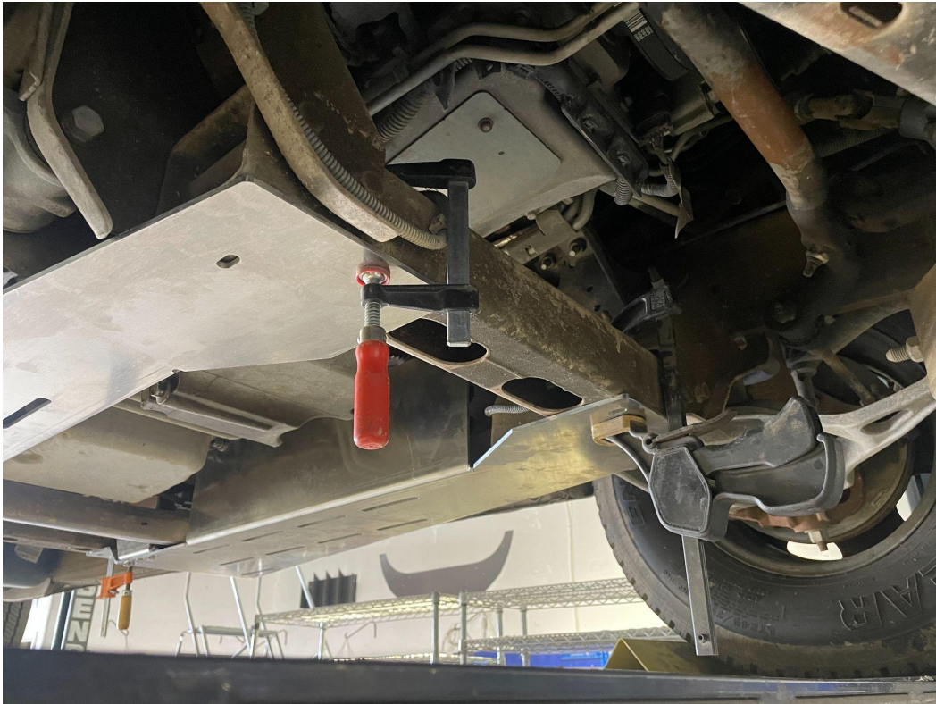
4.) Mark the 8 slots in the cat guard onto the frame.
