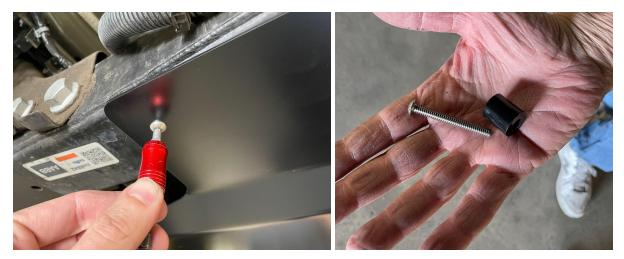
6.) Install your 5-16"-18 x 1" bolts/washers/**NYLOC** nuts through the slot(s) at the rear in the subframe (**2 bolts for STANDARD**, **1 bolt for TRAIL BOSS** / **AT4**). Point bolt(s) upward. **STANDARD**: Securely tighten all security bolts and 5/16" bolts/nuts.
