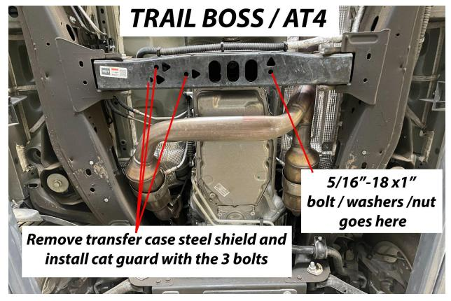
The **STANDARD** is shown here in the next pictures. **TRAIL BOSS / AT4** is the same process but the most rearward left hole will be omitted because it will be covered by the transfer case steel shield.
