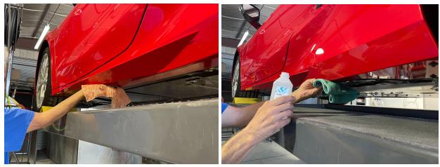
3.) Run 1 strip of double sided tape along the entirety of the rocker panel underside ( $\sim$ 78"). Keep it toward the outside of the rocker panel so the tape is about  $\frac{1}{8}$ " away from the edge. We represented this tape by a green line. Use pressure upward to firmly apply the tape.
