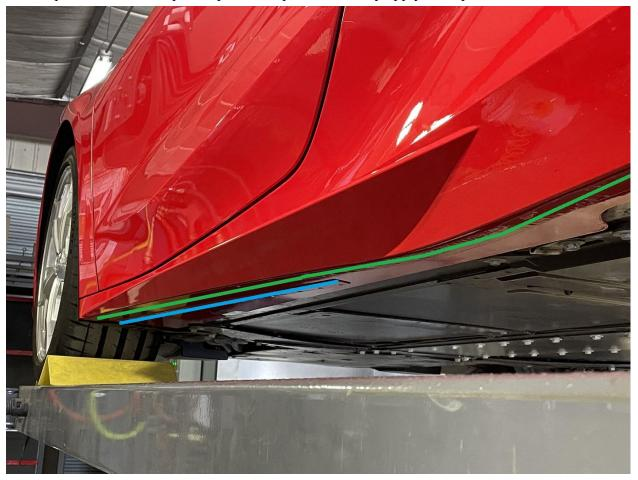
5.) Identify and remove the 3 screws found under the rocker panel on the car. There is 1 at the front, and 2 at the back. Use your ratchet wrench and 7mm socket. **REAR SHOWN HERE:**
