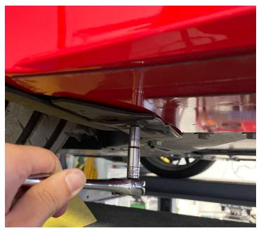
6.) Install a side skirt extension onto the rocker panel using the screws just removed. The side skirt extension will need to be slipped above the black plastic at the front so it sits entirely against the rocker panel.
