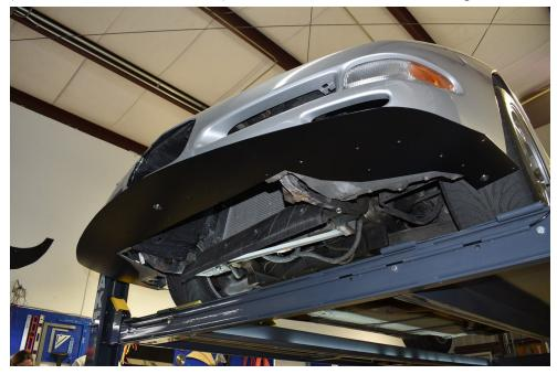
7.) Drill through the remaining holes in the splitter into the front bumper. Hold it up against the bumper while doing so.
