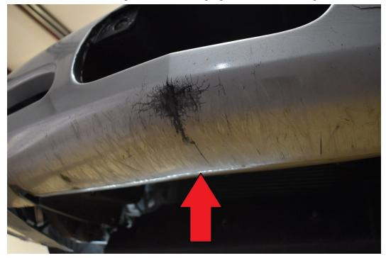
5.) Temporarily install your splitter onto the bumper into the holes from step three using M6-1.0 x 20mm bolts & 1" OD fender washers on bottom and  $\frac{1}{4}$ " small washers + m6 nyloc nuts on top. Make sure the splitter is centered and mark through the center hole in the splitter onto the front bumper with masking tape. Remove the splitter and drill a hole at the marked location using your  $\frac{1}{4}$ " drill bit.
