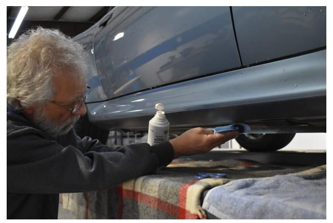
5.) Install one of your side skirts into the rear 4-5 holes. They can only go one way. Let the front hang down. Peel off the tape lining and push the skirt up against the tape then install the front 4-5 bolts remembering that the front hole has a longer bolt.
