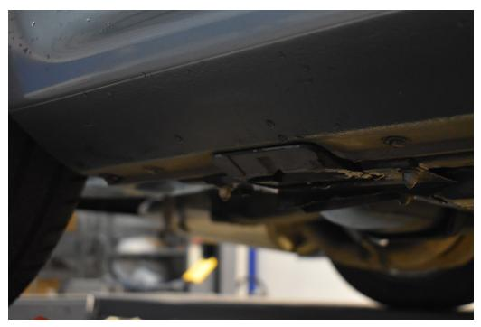
4.) Thoroughly clean the underside of the rocker panel where the side skirt will mount. Use the cleaning products and isopropyl alcohol to assure there is no dirt left. Then apply 3M tape along the ENTIRE flat portion of the rocker panel. It may need to be cut into sections around the jacking areas. Do not cover the bolt locations, and do not peel away the bottom side of the tape yet. (2 PICS)
