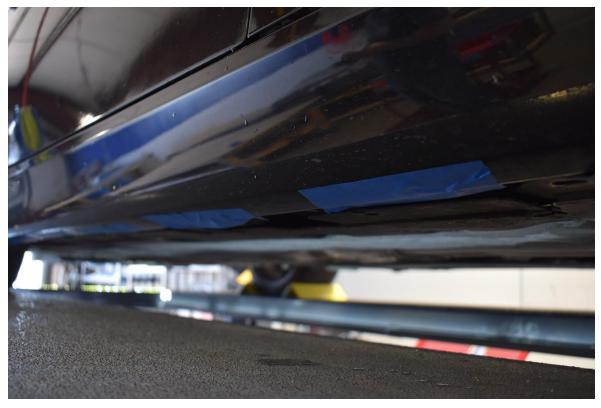
3. Remove the plastic undertray to the inside of the rocker panel. There will be several T30 screws, 10mm plastic nuts, and 8mm screws holding it on. (3 PICS)
