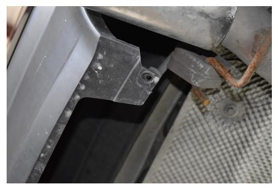
6. DIFFUSER TIME. With help from a friend install your diffuser onto the 3 installed brackets toward the front of the car. Use two M6-1.0 x 20mm bolts, two 1" OD fender washers (on the bottom), two small washers (on the top), and two nyloc nuts to install the diffuser onto the squared bracket. Use the same bolt/nut/washer set up for the hanger brackets EXCEPT INSTEAD use small washers on the bottom instead of the 1" fender washers. Point bolts upward and tighten securely. (3 pics)
