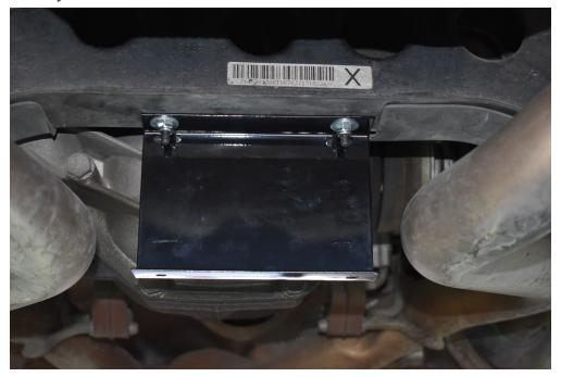
4. Identify the holes found in the left and right brackets on the frame of the car (not sure what to call these things but they have L (left) and R (right) indications. Insert a M6-1.0 through each hole and attach the supplied hanger brackets (as shown, 4 pics) on the appropriate sides using small washers and nyloc nuts. DON'T tighten all of the way. Allow for some minor rotation.
