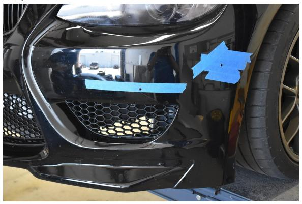
5. Remove the tape and install your canard using the supplied countersunk allen head bolts/washers on the outside, rubber washers in between the canard & car, and ¼" small washers & nyloc nuts on the inside. Apply the edge trim on top with the short end hanging inward toward the car before tightening fully - it acts as a cushion between the canard and the car. Tighten the bolts securely. (see 2 pictures!)
