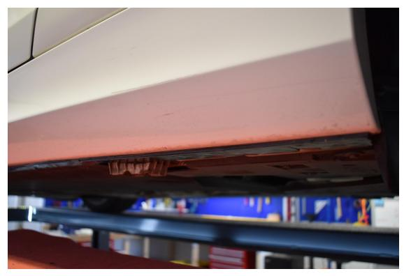
5. Install your skirt starting with the rear hole and moving forward. If any bolts don't want to install, skip them. We have a solution after you install the skirt. After your bolts have been installed and the skirt is properly situated front-to-back, push the skirt up onto the tape *firmly* and make sure it sticks across the entire length.
