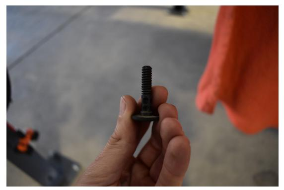
3. Temporarily install the skirt onto your car using these bolts just removed. These bolts do not, and cannot, be tightened too much. By temporarily installing the skirt you will get an idea of where you will be placing double sided-tape under the rocker panel, will allow you to check to see if all bolts will go back into their holes without popping out, and help you find where the skirt sits front-to-back.
