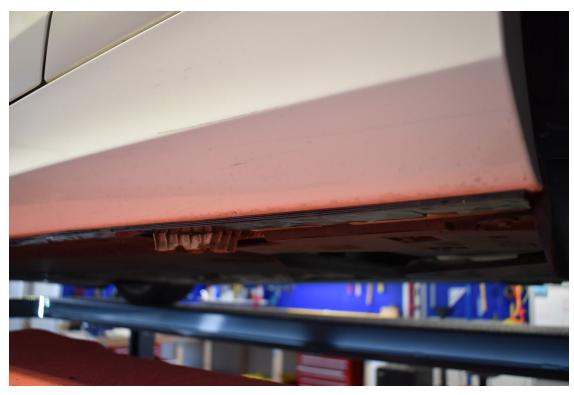
5. Install your skirt starting with the rear hole and moving forward. If any bolts don't want to install, skip them. We have a solution after you install the skirt. After your bolts have been installed and the skirt is properly situated front-to-back, push the skirt up onto the tape *firmly* and make sure it sticks across the entire length.
