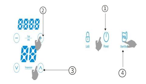
**NOTICE:** Long press the "Start/Stop" button for 2 seconds can reset the unit to the default state of 55°C / 131°F and 150 mL water output volume.
